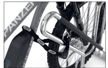
The 4801 XXBF parker with frame rest offers a parking space for bicycles with up to 70 mm wide tyres, which means that even bicycles with extra-wide tyres can be parked safely. The safety of the bicycle is guaranteed: The plastic impact protection protects the bicycle frame from damage. The leaning bracket ensures that the bicycle cannot tip over, and round steel eyelets serve as attachment points for bicycle chains. The bicycle stand is prepared
